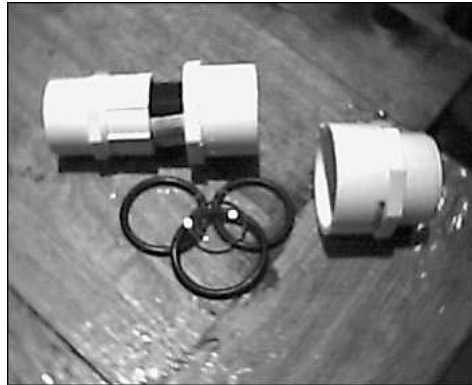
Figure 10 – Assemble the negative eyepiece using the double concave negative lens
