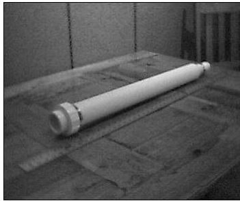
Figure 1 - Mailing tube refractor built from this handout. Focal length: ~ 38" (97cm) for a negative lens and 48" (121cm) extended for a positive lens; Aperture: ~ 2" or 50mm
