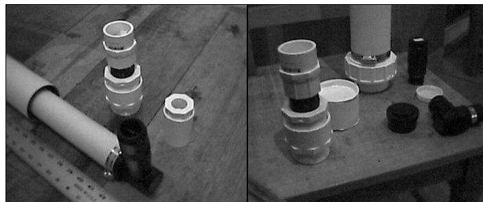
Figure 2 – Negative (Galilean) and Positive (Keplerian) PVC eyepieces and a stock 2" to 1 1/4" telescope adapter with right angle and 40mm lens
